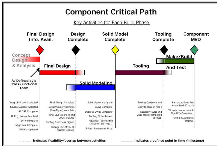
Exhibit 1. Sample Illustration of a Simplified Component Critical Path
